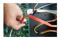
5. Use the special data cable to connect the HDD and the SATA port
